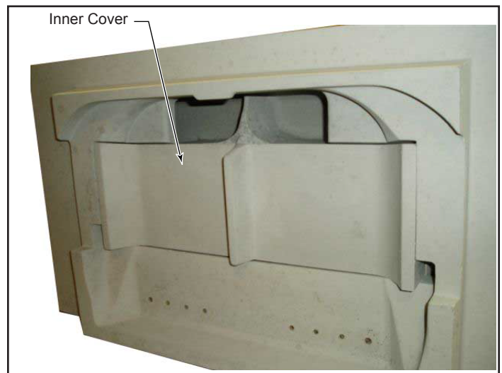
Figure 29 - Remove inner cover.
